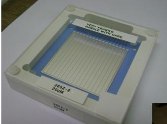
Detector telescopes: 50 x 50 mm<sup>2</sup> 20  $\mu$ m SSSD + 1000/500  $\mu$ m PSD & DSSD Particle identification from p to <sup>12</sup>C
