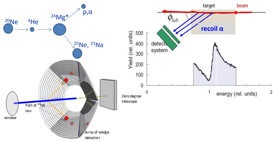
Fig. 3. The proposed experimental arrangement to be placed within the gas volume.
