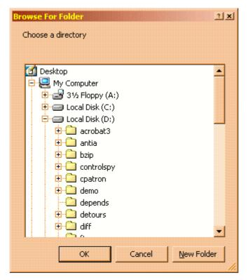
If the call worked, i.e. if the user interface returns a valid pointer and not NULL, we should translate the meaningless stuff we receive into a real path, so we call SHGetPathFro-mIDList, to do exactly that. We pass it a pointer to the result character string that we receive as second argument.
