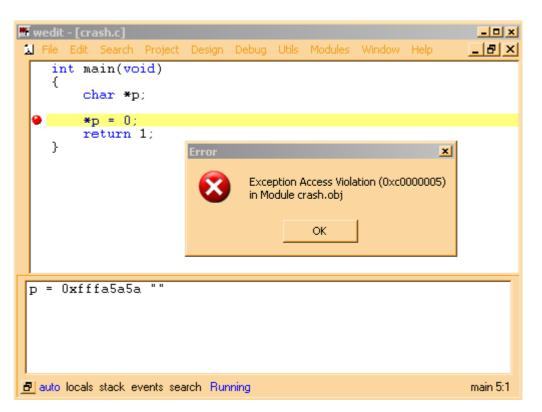
The debugger tells us that a machine exception has occurred, with the code 0xc0000005. This means that the CPU has detected an invalid memory reference and has called the exception mechanism of windows, that notified the debugger of the problem. Note the value of the pointer in the output window: 0xfffa5a5a.
