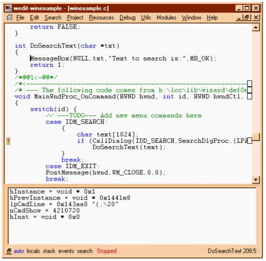
Our program starts running, we go to the menu, select the search item, and Wedit springs into view. We hit the breakpoint. Well that means at least that we have correctly done things until here: the message is being received. We enter into the CallDialog procedure using the F8 accelerator. We step, and after going through the DialogBoxParam procedure we see no dialog and the return result is -1. The debugger display looks like this:
